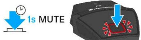
If the boundary microphone is on, press the ON/OFF button for 1 second.
