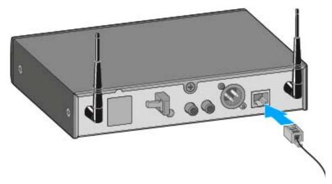
▷ Connect the other end of the network cable to a router or a switch.
