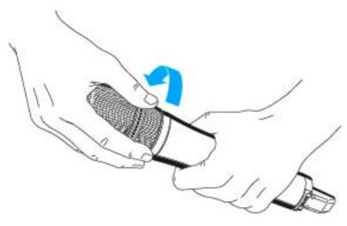
The microphone capsule can be unscrewed and replaced by one with a different pick-up pattern.
