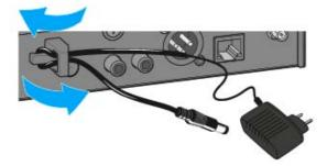
▷ Connect the hollow jack plug of the power supply unit to the DC IN socket of the receiver.
