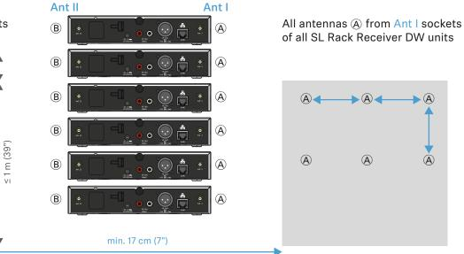
When using multiple AWM 2/AWM 4 antenna wall mounts, make sure that the distances between all antennas are equal:
