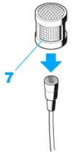
An additional frequency response cap (MZC 1) is available as accessory. The MZC 1 ensures a treble boost of 2 dB.
