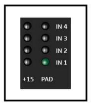
The PAD LED of the IN 1 input lights up: PTP Slave, with PTP Sync
