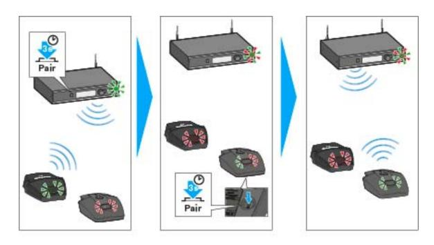
Once the radio link is successfully established, **Paired** appears on the display panel of both the receiver and the transmitter (only for SL Handheld DW and SL Bodypack DW) and the status LEDs on the transmitter and the receiver light up green.
