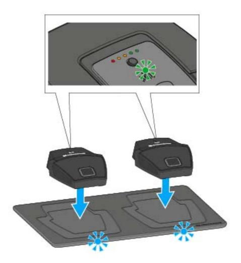
Place the boundary microphone on the CHG 2W charging base in the area marked.
