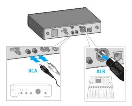
Use a suitable audio cable to connect the amplifier or the mixing console to the appropriate audio output of the receiver.
