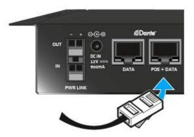
Use an Ethernet cable (CAT-5 or higher) to connect the POE + DATA socket of the SL DI 4 XLR to a PoE port of a PoE-enabled network device.
