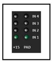
The PAD and the +15 LED of the IN 1 input light up: PTP is being synchronized.
