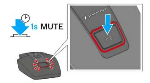
While the table stand is switched on and a goose neck microphone is connected, press the ON/OFF button for 1 second.
