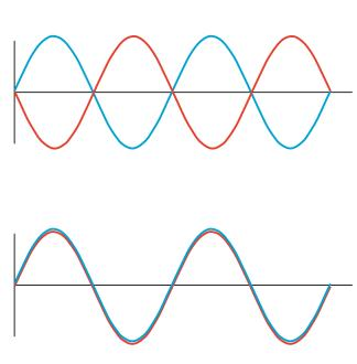
The signal is reflected by the electrically conducting surface. At worst, the blue signal and the red reflected signal are out of phase when they reach the receiver so that the two signals cancel each other out.
