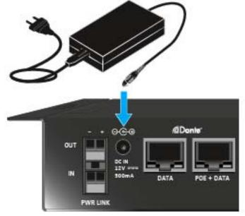
Connect the NT 12-50CS power supply unit to the DC IN socket of the SL DI 4 XLR.
