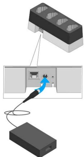
▷ Guide the cable through the cable guide at the base of the charger so that the charger is stable once in position.
