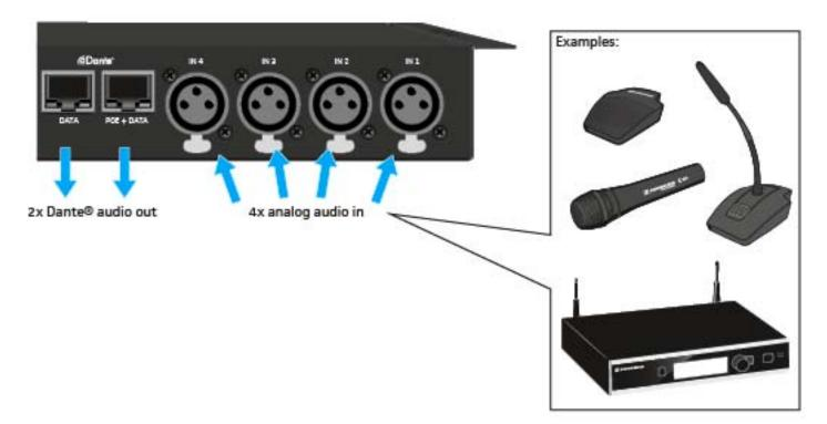
Via the DATA and POE + DATA Ethernet sockets, the audio signals are routed, using Dante<sup>™</sup>, to a Dante<sup>™</sup>-enabled device.
