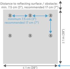
If possible, position the antennas so that there is a direct line of sight (without obstacles) between the transmitters and the antennas.
