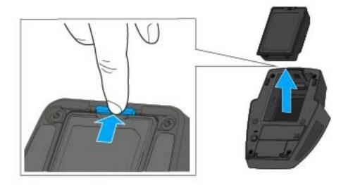
▶ Pull the unlock button away from the accupack and pull the accupack out of the compartment.
