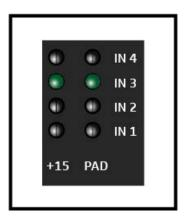
The +15 LED of the IN 3 input lights up: Memory Stack Overflow
