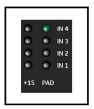
The PAD LED of the IN 4 input lights up: System is ready for operation
