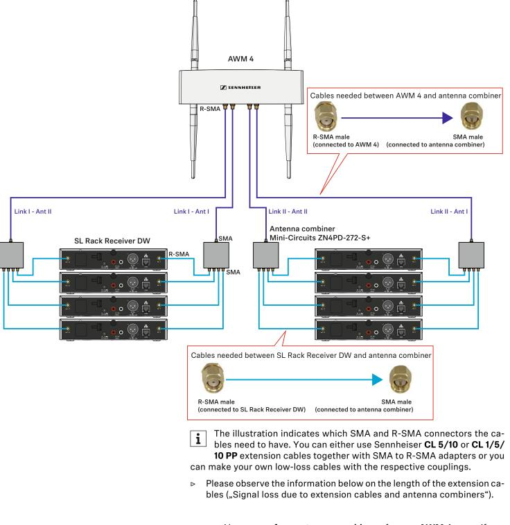
Always use **four antenna combiners** for **one AWM 4**, even if you use fewer than eight receivers. Always combine all antenna sockets ANT I of up to four receivers and all antenna sockets ANT II of up to four receivers respectively to the two sockets of one link of the AWM 4. If you are not using all antenna sockets of the antenna combiner, lock the unused sockets with a terminating resistor (50  $\Omega$ ) to reduce incoming interference and to maximize the RF performance.
