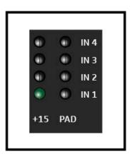
The +15 LED of the IN 1 input lights up: PTP Error / No PTP Sync / PTP deactivated
