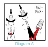
**NOTE:** The provided wire nuts are meant for permanent installation use only. If you are temporarily wiring the speakers, do not use these wire nuts. In the event you have used the wire nuts, and need to re-wire your system, do not attempt to unscrew the nuts. Instead, clip the wires below the nut, and follow the steps in the Basic Wiring section with a new pair of waterproof wire nuts (these are available at most hardware stores).
