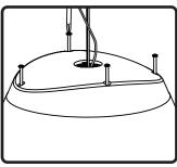
11. Tighten all four (4) screws to lock cover plate in place.
