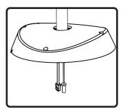
4. Run RJ45 signal wire and at least one safety cable through conduit.
