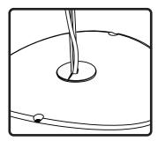
12. Install rubber weather plug by sliding slit over the wire, then pressing snuggly into hole in cover plate.
