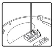
7b. Once aligned with central slot, pull cable up into slot to secure. Repeat steps 7a and 7b with secondary safety cable into one of the side slots.
