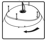
10. Place cover plate onto top of speaker and rotate clockwise until alignment indicators meet.
