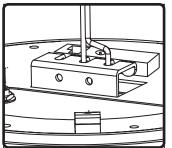
8. Extra slot and 2 holes provided for additional safety cables where needed.
