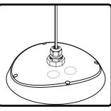
4. Tighten the top of 3/8" NPT wire gland such that the rubber grommet is tight around the cable. This may require a wrench.
