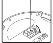
6. Align safety cable with center slot and pull up to secure.
