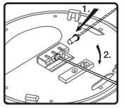
5. Attach safety cable by first inserting into side of mounting bracket.
