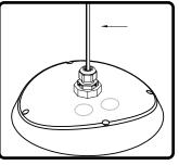
connector, through the 3/8" NPT wire gland and attach to the back of the speaker as noted in previous instructions.
