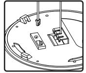
7. Plug RJ45 connector into speaker. If local power\* is required at speaker (non-POE appropriate DC power supply to barrel connector on speaker input panel.
