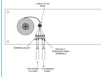
If transformers are being freely-mounted on a panel within an equipment rack, fit lockable side and rear doors, and blank 19" panels as necessary to the rack, to prevent access to the terminations. If the transformers are to be housed externally to a rack, the use of a lockable IP-rated enclosure fitted with the appropriate cable grommets is recommended.
