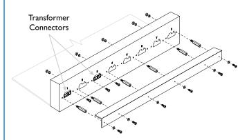
**IMPORTANT:** If less than eight transformers are installed in the rackmount housing, it is still important to fit all six hex pillars (supplied) in the positions indicated. If a connector position requiring a hex pillar is empty (due there being no transformer in that position), use an M3 shakeproof washer and nut (supplied) to secure the hex pillar in place.
