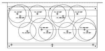
When each transformer position has been determined, insert the bolt from the underside of the chassis, place the transformer in position with the bolt through the central hole, and secure it in place with the washer and locknut supplied. Before final tightening, rotate the toroids to ensure that the cable assemblies for all the transformers emerge from the windings at a neat orientation for wiring to the rear panel.
