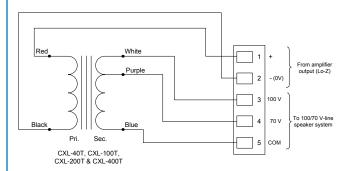
Each transformer has five colour-coded wires which terminate on a small PCB.A 2-way and a 3-way 5 mm-pitch female connector, and two M3 fixing brackets are fitted to the PCB. Locate the connectors into the rectangular rear panel slot which is in line with the transformer's position. Note that, looking at the rear panel, the 3-way connector goes to the left of the slot.
