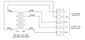
Each transformer has five colour-coded wires which terminate on a small PCB.A 2-way and a 3-way 5 mm-pitch female connector and two M3 fixing brackets are fitted to the PCB. Locate the connectors into the rectangular rear panel slot which is in line with the transformer's position. Note that, looking at the rear panel, the 3-way connector goes to the left of the slot.
