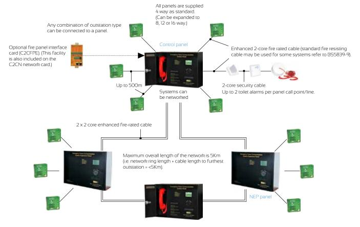
Up to 16 panels can be placed on the network (2 of these can be control panels, one of which will act as a slave unless activated as the master during an emergency).
